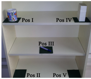
Fig. 1: Birdview of the experimental setup consisting of three (3) everyday life objects, a marker, a rectangle and a mug, placed on three (3) different shelves of a bookcase, in five (5) different positions
